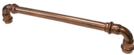
Copper connecting bend with press fittings Krantz-recommended component for interconnecting two adjacent KKS-4/GK elements at the standard spacing; factory-made to the required spacing and fitted with Viega press fittings (press contour V). Supplied on request.
