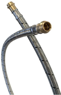
Flexible connecting hose with press fittings Krantz-recommended component for interconnections between KKS-4/GK elements outside the standard spacing and for the building-side connection to the heating/chilled-water system. Stainless-steel braid (AISI 304), oxygen-diffusion-tight to DIN 4726, with an extremely smooth inner surface for reduced pipework pressure losses; fitted with Viega press fittings (press contour V). Supplied on request.
